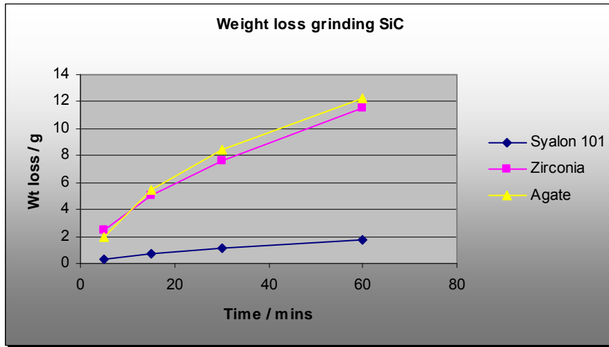
Fig. 2 Weight loss data for samples ground in mill Configuration 2
