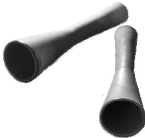
Traditionally liners have been made from tungsten carbide. However, at the low angle impacts encountered in many blasting operations, tungsten carbide nozzles wear excessively due to the erosion of the relatively soft and ductile cobalt used to cement the carbide grains together.
