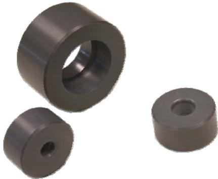
As a solid solution, the vapour pressure of  $\beta$ -sialon is lower than that of  $\text{Si}_3\text{N}_4$  and as a result the sialon will form more liquid at a lower temperature with  $\text{Y}_2\text{O}_3$ . Sialon is thus more easily densified using normal sintering techniques. Furthermore, it should be noted that the lower vapour pressure of sialon reduces decomposition at high temperatures so that the sialon is thermodynamically more stable than  $\text{Si}_3\text{N}_4$ .
