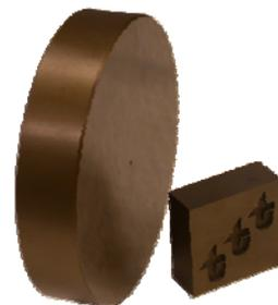
The first, **Syalon 501**, is based on  $\beta$ -sialon and is an electrically conductive grade which can be electro-discharge machined into complex shapes. It possesses many of the excellent properties of Syalon 101 and has found application as extrusion dies and die pressing dies.
