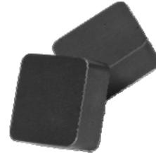
This demanding set of requirements is met by **Syalon 050**. It is thermally stable up to 1400°C, thermal shock resistant, hard, tough and strong and chemically resistant to corrosion. In use Syalon 050 cutting tips reduced by 75% the machining time for turbine discs for the Rolls Royce RB211 engine.
